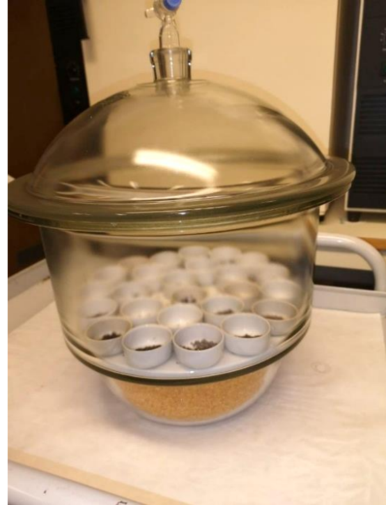
Figure 6: Desiccator with soil samples (Photo: Martina Vårdal)
