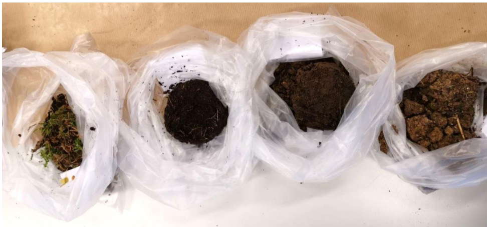
Figure 5: One soil sample divided into four layers (Photo: Martina Vårdal)
