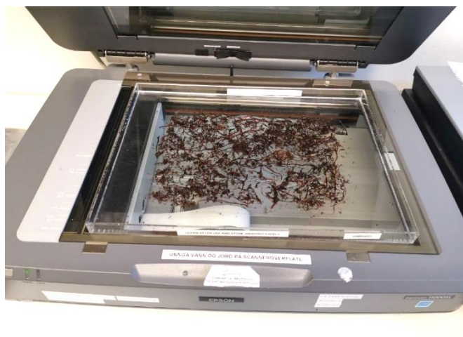
Figure 10: EPSON scanner with washed root sample (Photo: Martina Vårdal)
