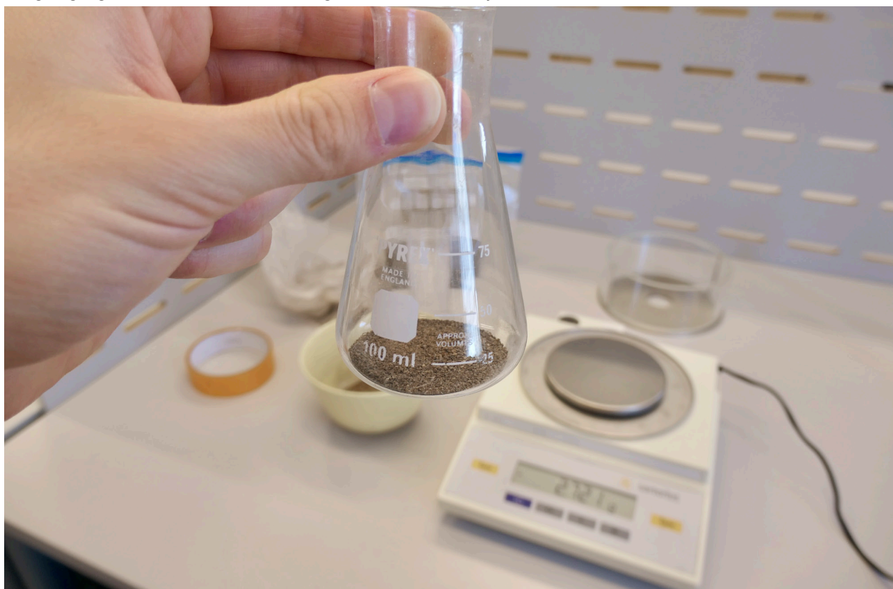
Weighing 5 grams of the soil before mixing it with the sodium hydroxide solution. Photo: Opitz, 2023.
