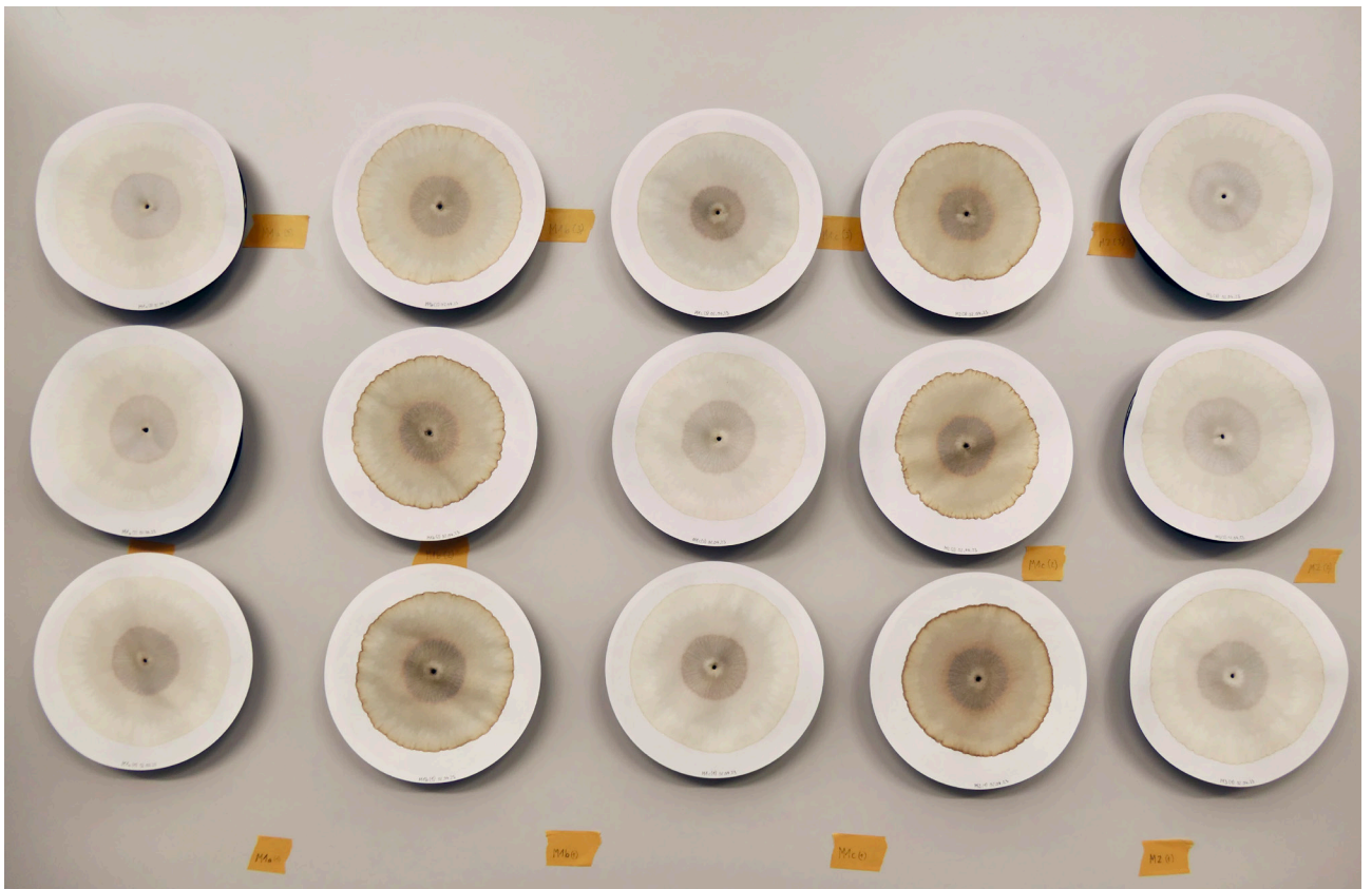
The chromatograms reflecting the Munich soil samples just after the experiment. Photo: Opitz, 2023.
