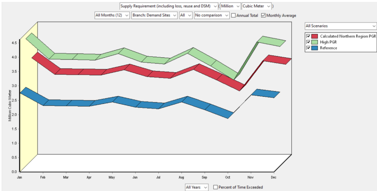
A.C Figure 87 - Monthly average of supply requirement for all years when there are two transmission links operating at maximum capacity, reduced loss rates and a reuse rate of 22.0%. Screenshot from the results view in WEAP.
