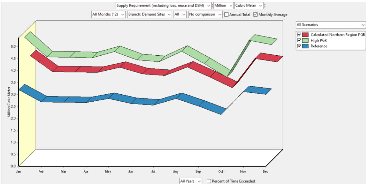
A.C Figure 63 - Monthly average of supply requirement for all years when there are two transmission links operating at maximum capacity and a reuse rate of 22.0%. Screenshot from the results view in WEAP.
