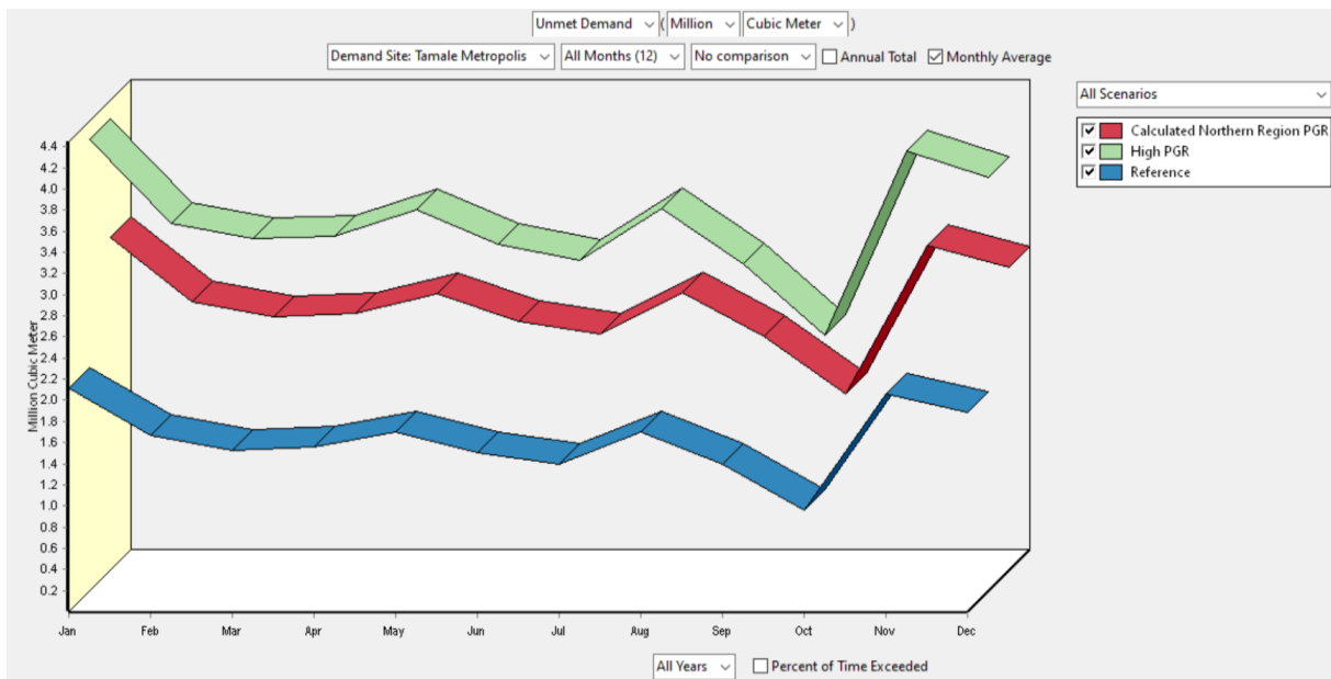
A.C Figure 84 - Monthly average for unmet demand for all years when there are two transmission links operating at maximum capacity and reduced loss rates. Screenshot from the results view in WEAP.
