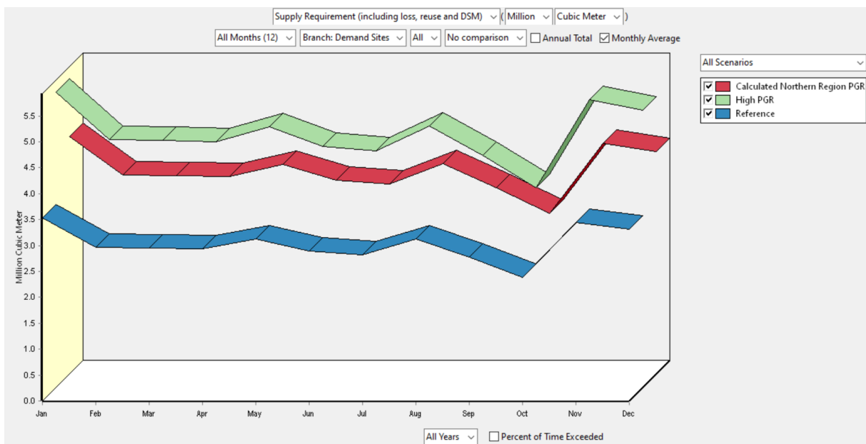
A.C Figure 82 - Monthly average of supply requirement for all years when there are two transmission links operating at maximum capacity and reduced loss rates. Screenshot from the results view in WEAP.
