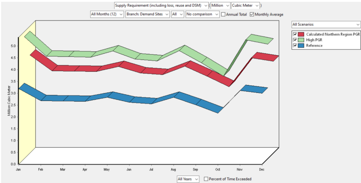
A.C Figure 57 - Monthly average of supply requirement for all years when the reuse rate is 22.0%. Screenshot from the results view in WEAP.
