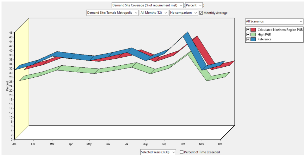
A.A Figure 35 - Monthly average of demand site coverage in 2030 for the scenarios in the PGR model. Screenshot from the results view in WEAP.
