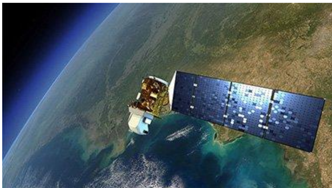
Figure 20 Landsat 8 Satellite Sensor with a 15m resolution [36]
