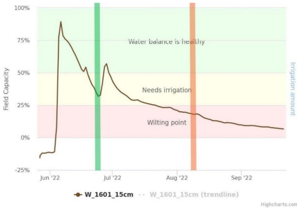
Figure 9: water balance recorded by one sensor in a dry section of the field in the elevated tunnel. The green marking highlights approximate timepoint for heading date, the red marking indicates the approximate timepoint for maturity.
