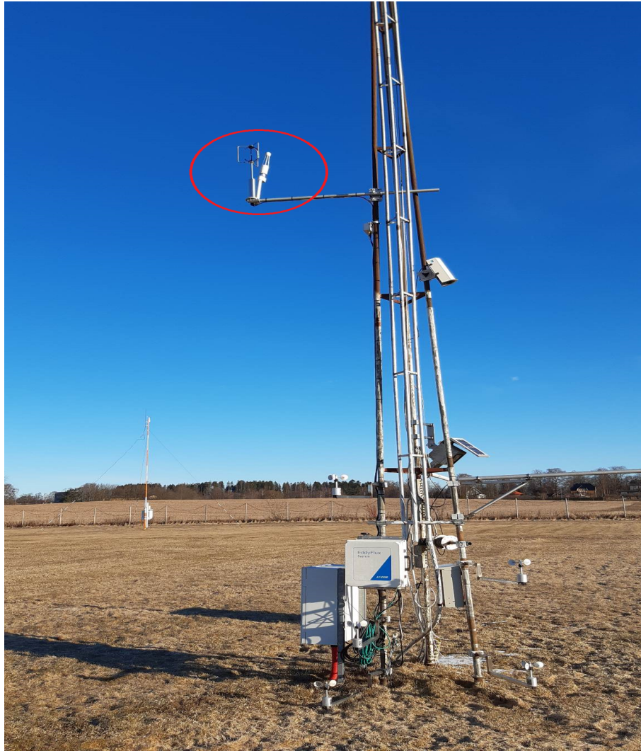
Figure 12: A picture of the eddy-covariance instrument (marked with the red ring) mounted on the eddy-flux tower.
