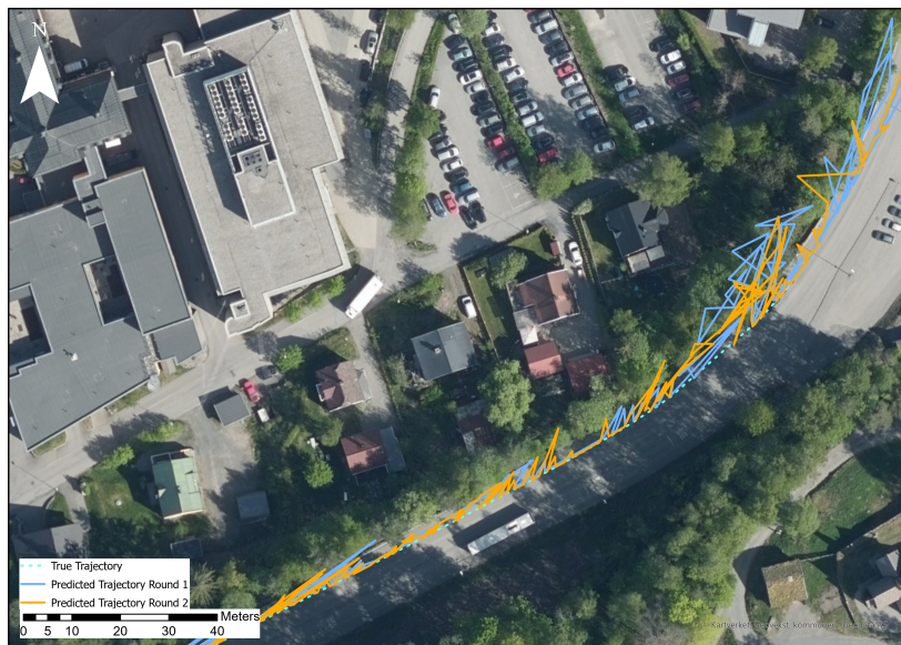
Figure 4.2.1: Visualisation of Round 1 and Round 2 in a forest area. Compared to the true trajectory. Background map from Kartverket, Geovekst, kommuner and Geodata AS (2023).
