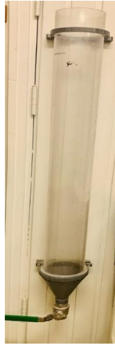
Figure 13: One-meter water column for measurement of sinking velocity
