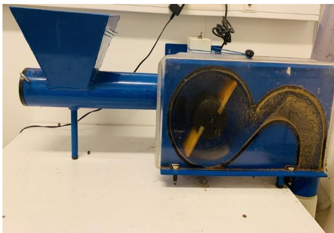
Figure 10: DORIS Pellet Tester shaker
