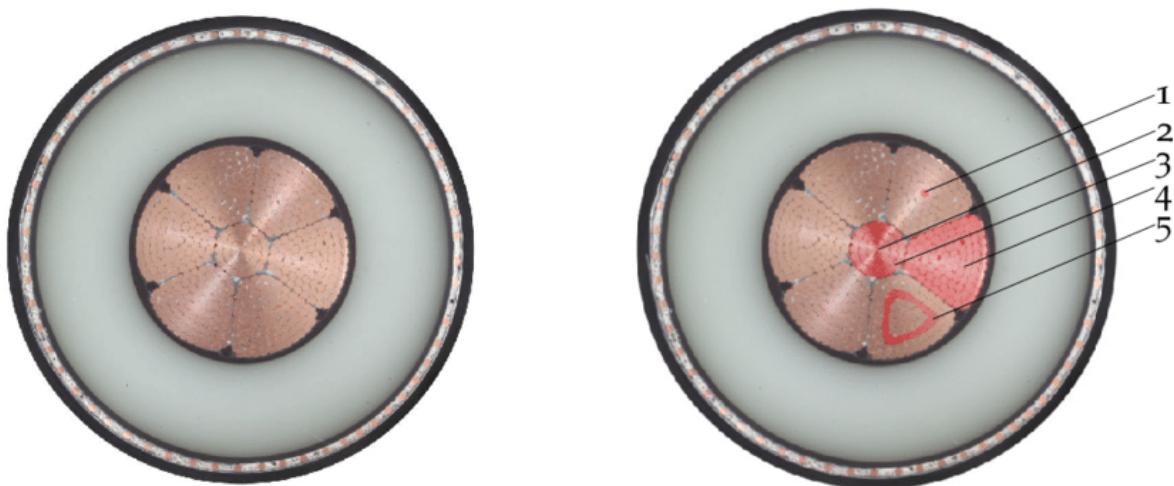
Figure 2.2: The figure shows a Milliken type conductor. The right portion highlights the details where the numbers represent: 1) single strand, 2) core of the cable, 3) one strand in the core, 4) segment of the whole conductor, 5) layer in a segment [17].
