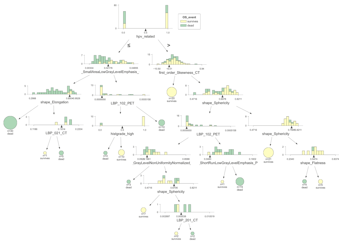
Figure 4.3.6: Tree 7 of 20 from the Random Forest model for predicting DFS on dataset DR3. Note that this tree is not the only tree that makes up the prediction of the Random Forest model. The prediction is made by a majority vote.
