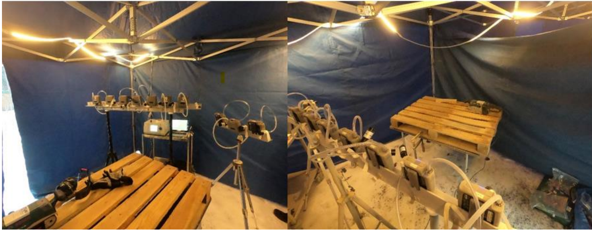
Figure 4: The pictures shows the set up inside the "workroom" where PM was produced with the pumps, real time collector, grinder and in this case the wooden material used to produce PM from wood.
