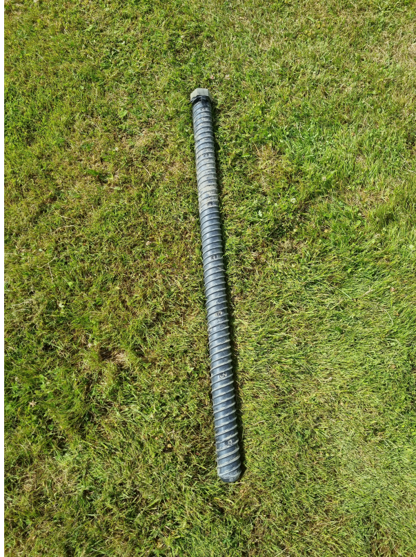
Fig. 9: SoilVUE sensor. Note the threaded design meant to optimize soil contact. Image from Laura Ehrnsperger.
