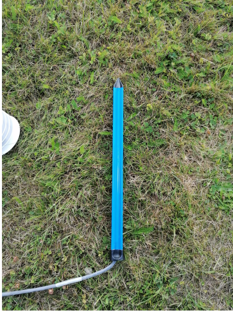
Fig. 12: The SMIoT sensor before insertion into the ground. Image from Laura Ehrnsperger.
