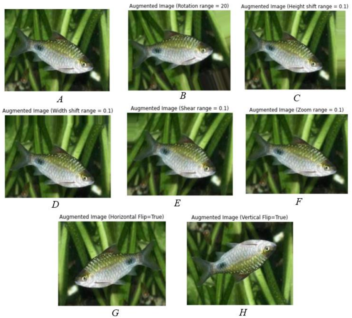
Figure 4: Various image augmentation methods. A: Original Image, other images are results of augmentation methods applied to original image. B: with rotation range 20, C: with height shift range 0.1, D: with width shift range 0.1, E: with shear range 0.1, F: with zoom range 0.1, G: with horizontal flip set as and H: with vertical flip set as true.
