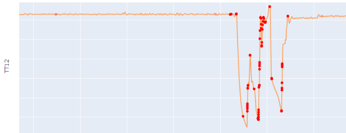
Figure B.31: Clog 3, anomalies detected using DBSCAN, showcased on TT12 sensor data
