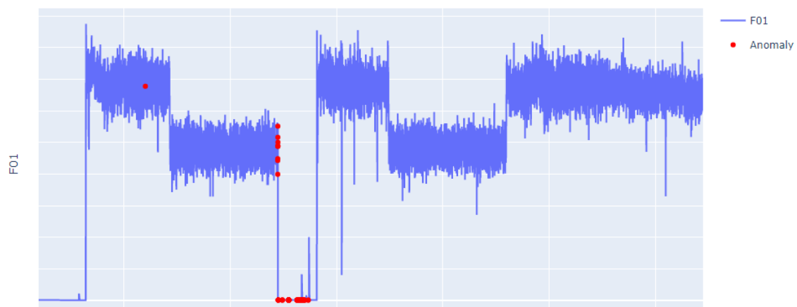
Figure 5.7: Clog 1, anomalies detected using DBSCAN, showcased on F01 sensor data
