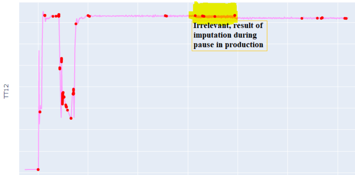
Figure B.10: Clog 4, anomalies detected using LOF on unfiltered data, showcased on sensor TT12
