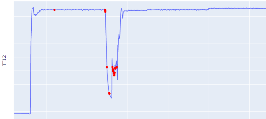
Figure 5.8: Clog 1, anomalies detected using DBSCAN, showcased on TT12 sensor data
