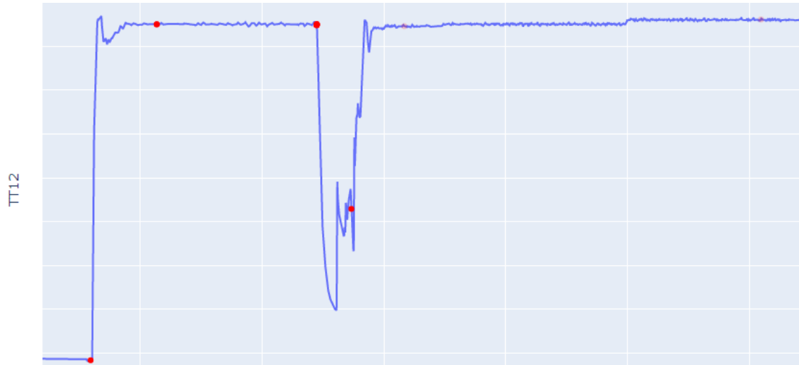
Figure 5.2: Clog 1, anomalies detected using LOF, showcased on TT12 sensor data
