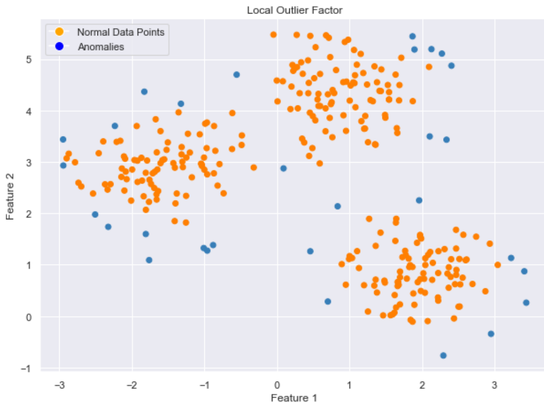
Figure 2.17: Application of LOF on randomly generated data
