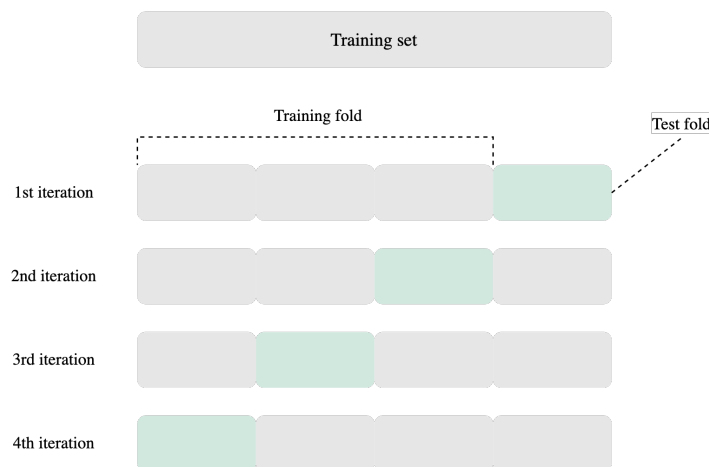
Figure 2.8: Illustration of a 4-fold cross-validation. The green boxes represent the test folds, whereas the gray boxes are the training folds. Illustration inspired by [17].
