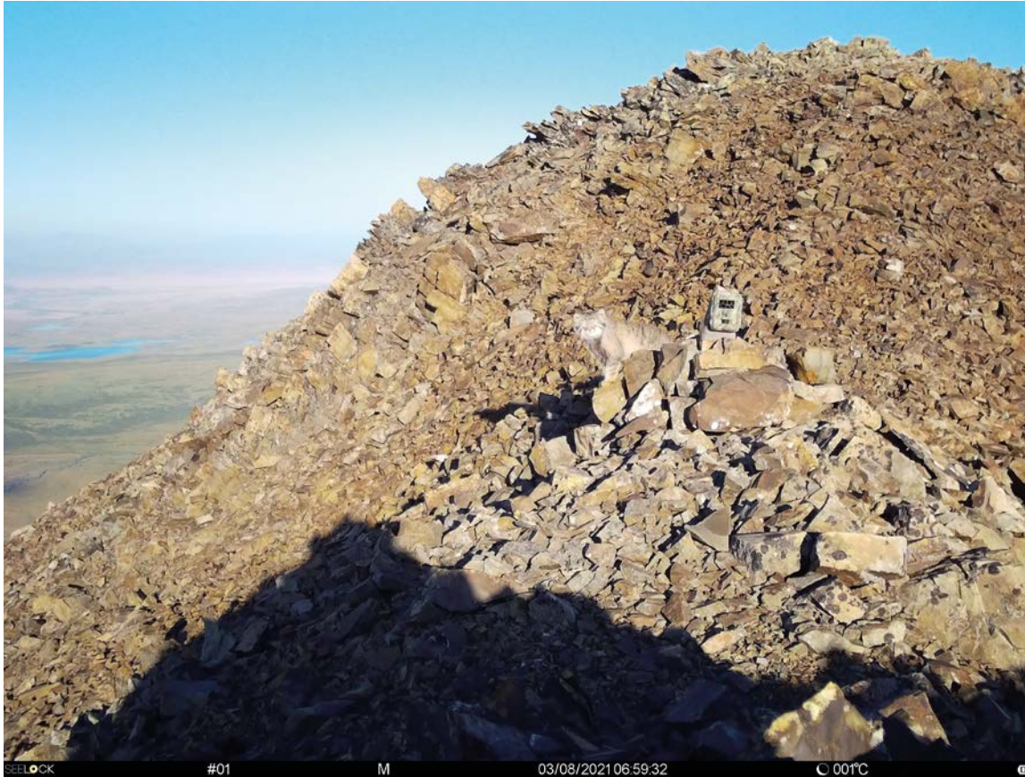
Figure 18: Paired cameras opposing each other should be directed towards the same focal point but not facing each other directly, otherwise they may trigger each other or result in overexposed images when the flashes are activated. Photo: S. Spitsyn/Altai Biosphere Reserve
