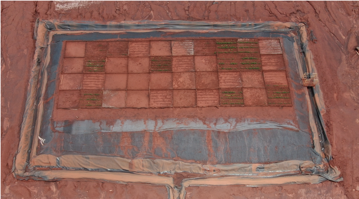
Figure 4.1: A drone photography of the pilot project from which the samples were collected. Each plot measured 9 m 2 and contained 2700 kg of bauxite residue mixed with amendments.
