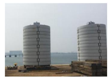
Figure 2.12: Gravity anchors (Group, n.d.)
