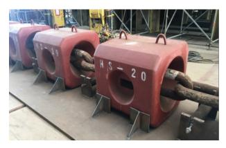
Figure 2.8: Clump weight from (Ma et al., 2019)
