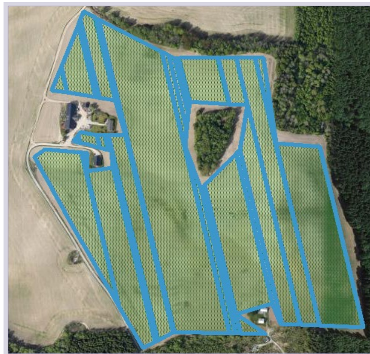
Figure 28: By converting the curved sides of the ROIs into straight lines with better size and smaller in number of sub-shapes will be produced. Which will have better sizes each to design many paths. The smaller they get in their number, the sub-shapes will create path discontinuity less often.
