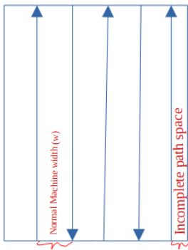
Figure 12: Normal machine width( w ) vs incomplete path space in path planning of a sub-shape.
