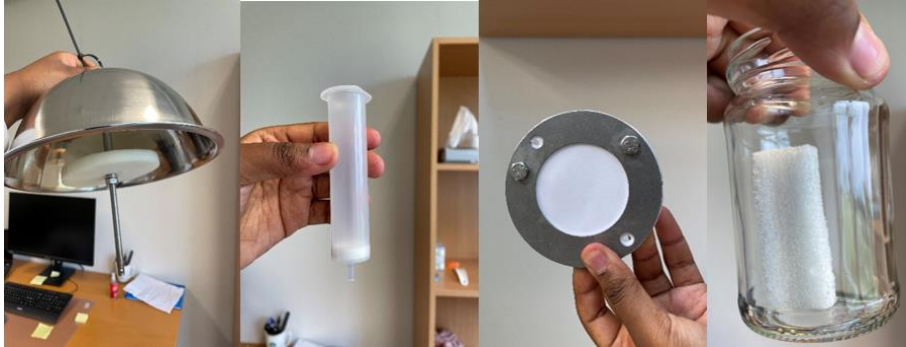
Figure 1 This figure shows a close up image of the PUF, ABN in Cartridge, POCIS and PDMS in that order.
