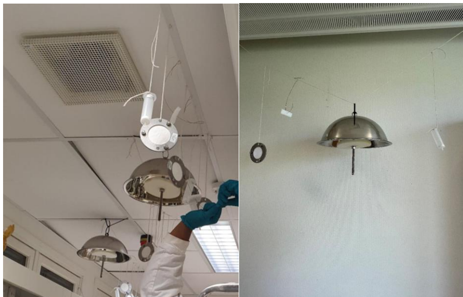
Figure 2 Deployment of ABN in cartridge, POCIS, PDMS and PUF. Right side shows the actual deployment, and the left side shows a model deployment.
