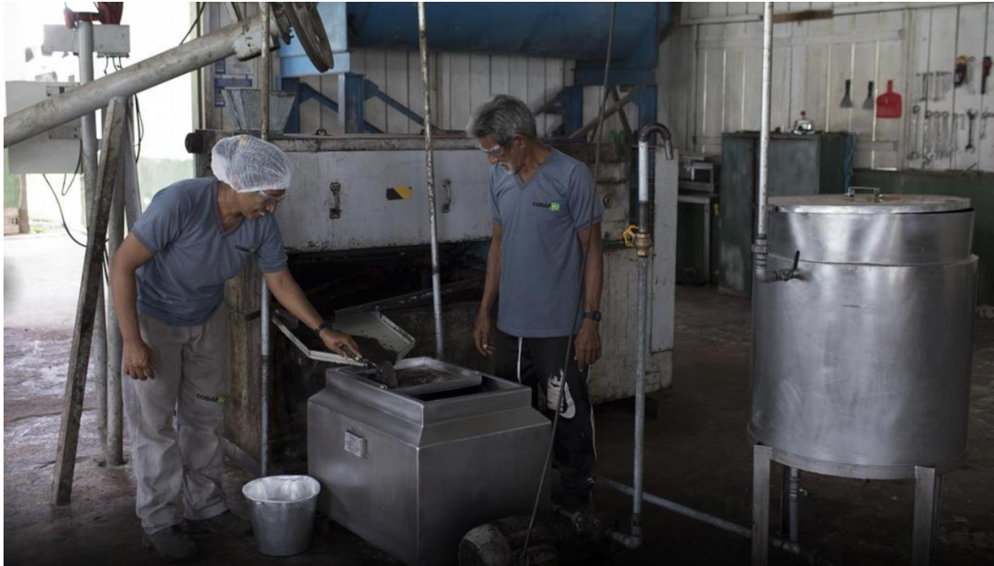
Figure 19: Oil Being Filtered at Roque's Processing Unit
