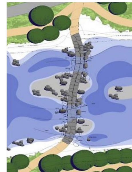
Figure 17e and 17f: For large machines to cross the river, they designed a threshold functioning as a road (Image source: Økogrønt, 2022).
