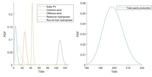
Fig. 5. Modelled range of generation levels for different technologies (left) and total production (right) in Norway.
