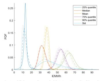
**Fig. 8.** Modelled mean, median, standard deviation and quantiles of the yearly price distribution in Norway. The solid line represents the 3 GW scenario, the stippled line 5.5 GW, and the dotted line 8 GW.
