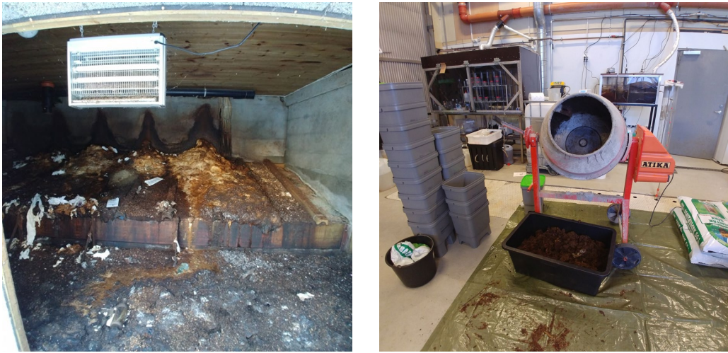
Figure 3. Left – the dry toilet collection compartment. Right – Mixing the substrates in a cement mixer.
