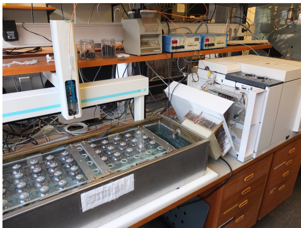
Figure 2. Photograph showing the robotized incubation system at the time of experimentation. Shown are (from left to right) the temperature-adjustable water bath with submersed magnetic stirring boards allowing simultaneous incubation of 30 120ml serum bottles and 10 non-stirred standard bottles, the peristaltic pump, and the gas chromatograph (GC). The robotic arm samples the bottles periodically (here 4 hourly) by piercing the crimp-sealed butyl septa of the bottles with a hypodermic needle. Ca. 1 ml of headspace gas is transferred with a peristaltic pump to a multi-column, multi-detector GC with loop injection for analysis of N_2 , O_2 , CH_4 , CO_2 and N_2O and a chemiluminescence analyser for analysis of NO (not shown). Upon injection, the pump is reversed, and unused sample is pumped back into the bottles together with helium, keeping flask pressure at \sim 1 atm. The resulting dilution is corrected for as outlined by Molstad et al. (2007). For a detailed description of the setup, see Molstad et al. (2016).
