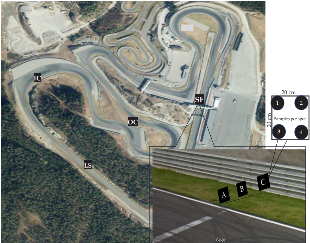
Fig. 1 Overview of the Rudskogen racetrack with sampling locations; start/finish (SF), long straight drive (LS), inward curve (IC), and outward curve (OC). The large insert (picture) shows the three different sampling distances from the edge of
