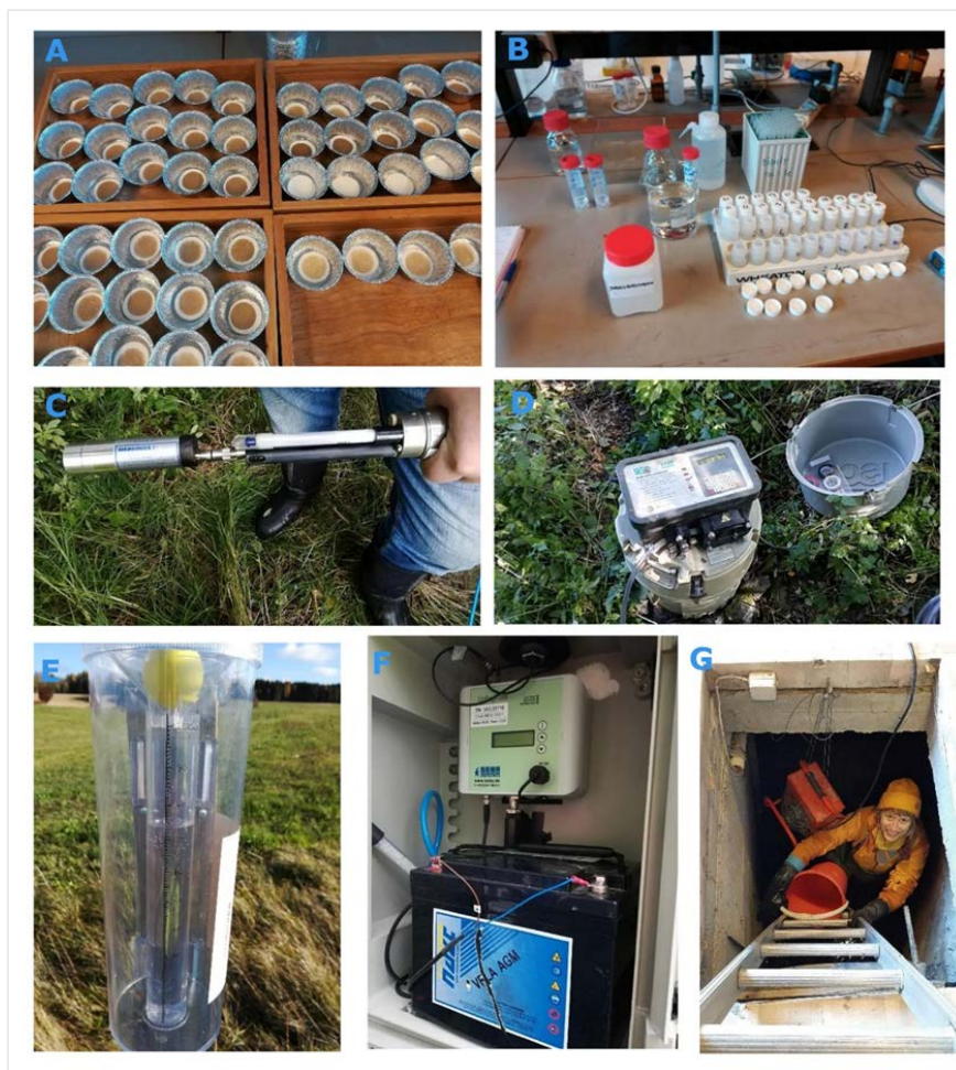
Figure 3: Impressions of field and laboratory work. A: filter papers with sediments after filtering the water samples, B: preparation of the phosphorus analysis, C: high-resolution turbidity sensor, D: ISCO portable sampler, E: rain gauge with tennis table ball to prevent evaporation, needed for isotope sampling, F: data logger of the turbidity sensor powered by a car battery; G: on the way to clean the turbidity sensor in Mørdre.
