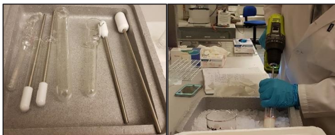
Figure 45. Potter-Elvehjem homogenisers and Dounce glass tissue grinder (left panel) used for the preparation of salmon liver microsomes (right panel).
