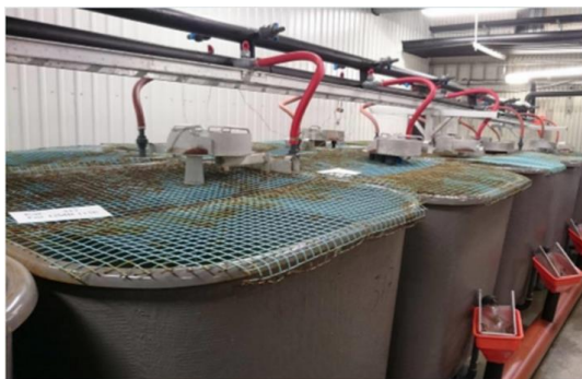
Figure 31. Salmon research tanks with automatic feeders and excess water collectors at Nofima, Sunndalsøra, Norway.
