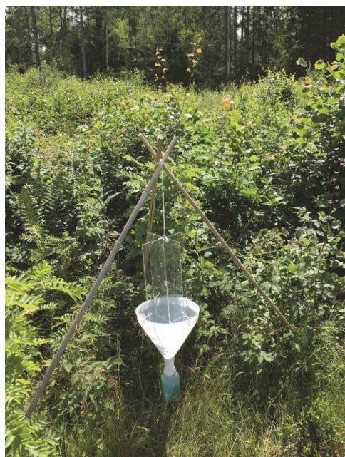
Figure A1: Photo of a flight interception trap in one of the sites in 2015. Photo: Mari Steinert.
