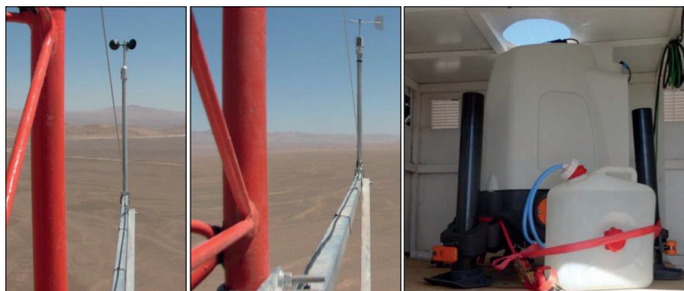
Figure 2.8. Instruments utilized at the CL site. Left and center panels: Anemometer and wind vane, respectively, mounted in a meteorological mast. Right panel: Deployed LiDAR. Courtesy of Mainstream Renewable Power.
