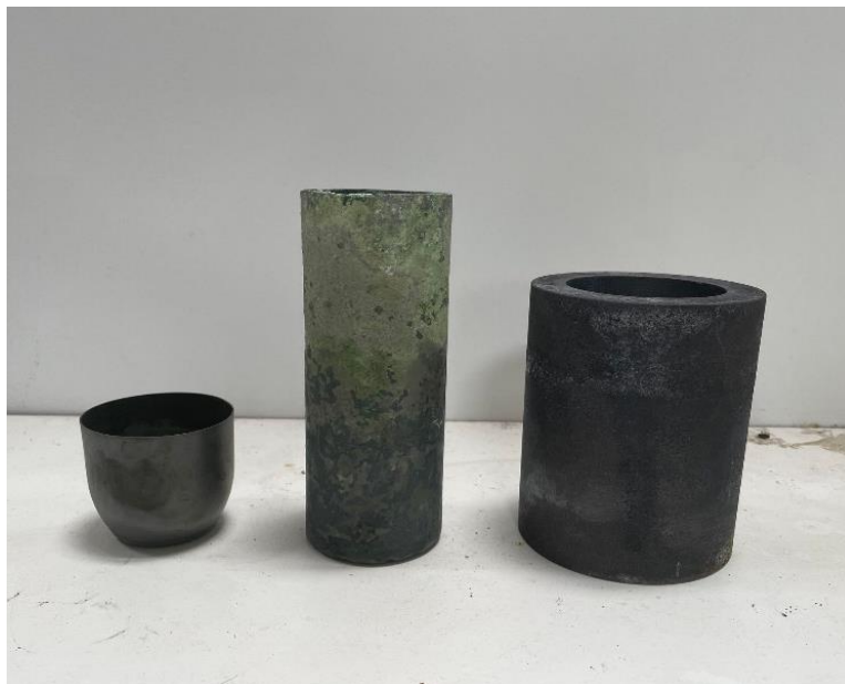
Figure 4.6. Crucibles used in different experiments from the left side: nickel crucible for melting point experiments, nickel crucible for TGA and hydrolysis experiments, and graphite crucible for electrolysis experiments.
