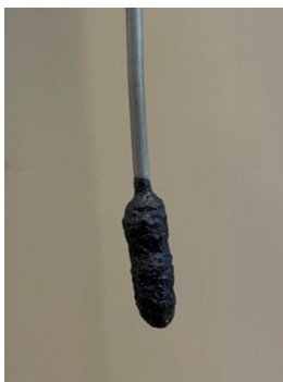
Figure 14. The deposited Mn from \text{MnO}_2 in the molten salt after 1.5 h of electrodeposition.
