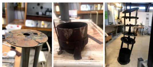
Fig. 8. The corrosion of the nickel radiation shields, nickel crucible containing molten salt and nickel stainless steel setup containing KCl-CuCl molten salt after an experiment in temperature range of 50-350 °C under inert atmosphere.
