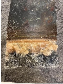
Figure 12. Cross-section of the crucible after 2.5 h electrodeposition of Fe from FeCl_3 in ZnCl_2:KCl:NaCl showing two separate layers, molten salt on top and Fe compound at the bottom.
