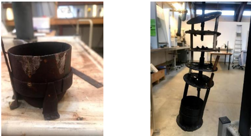
Figure 5.11. The corrosion of the nickel crucible containing molten salt and nickel stainless steel setup containing KCl:CuCl molten salt after an experiment in a temperature range of 50–350°C under an inert atmosphere.
