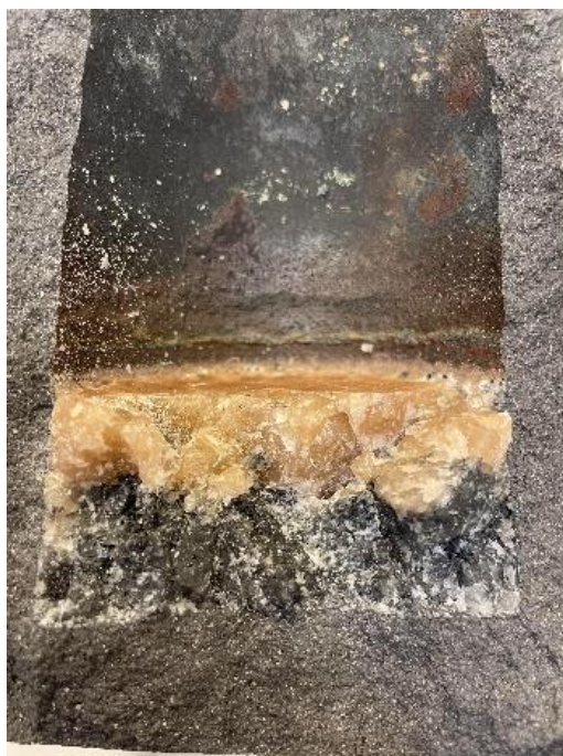
Figure 5.15. The cross section of the crucible after 2.5 h electrodeposition of Fe from FeCl_3 in ZnCl_2:KCl:NaCl showing two separate layers: molten salt on top and Fe compound at the bottom.
