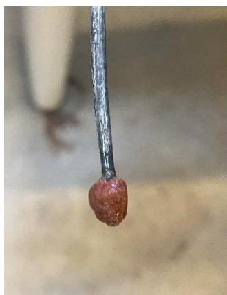
Figure 5.14. The deposited (a) Cu from CuCl and (b) Mn from \text{MnO}_2 in the molten salt after electrodeposition.
