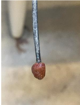
Figure 8. The copper deposited from CuCl in the molten salt after 1.5 h of electrodeposition
