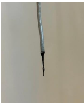
Figure 15. The Zn electrode after a few minutes potentiostatic experiment in \text{ZnCl}_2\text{:KCl:NaCl} containing \text{MnO}_2 at 360\text{ }^\circ\text{C}
