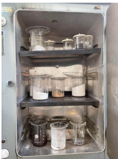
Figure 4.1. Beakers containing different salts kept inside the heating cabinet at a temperature of 200^\circ\text{C} .
