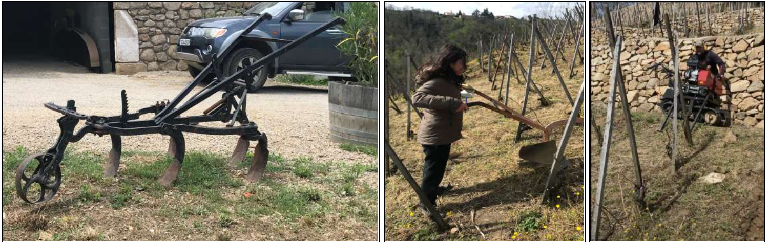
Figure 9. A mechanical weeding plow (left). Anna working the plow attached to a motorized pulley ( treuil ) along the vines (center). A worker operating a motorized pulley positioned at the top of the row to be weeded (right).
