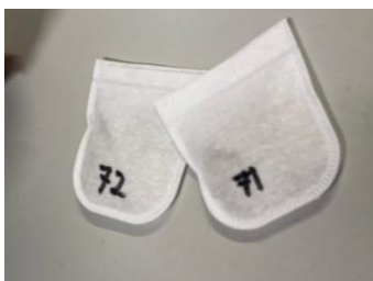
Figure 22. The Ankom F57 filter bags with feed
