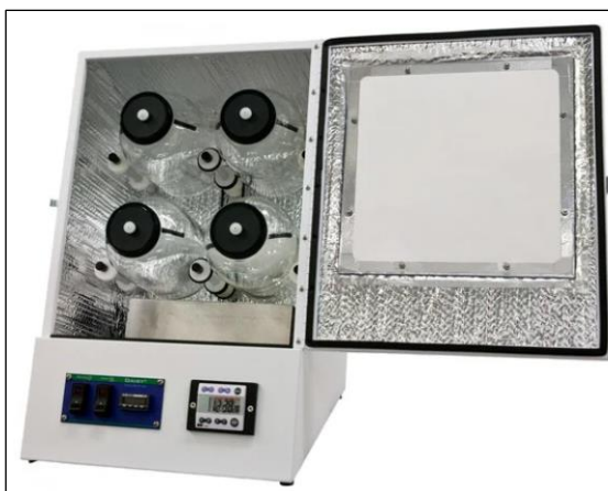
Figure 13. The ANKOM Daisy incubator with four digestion jars. From (ANKOM, n.d -b)
