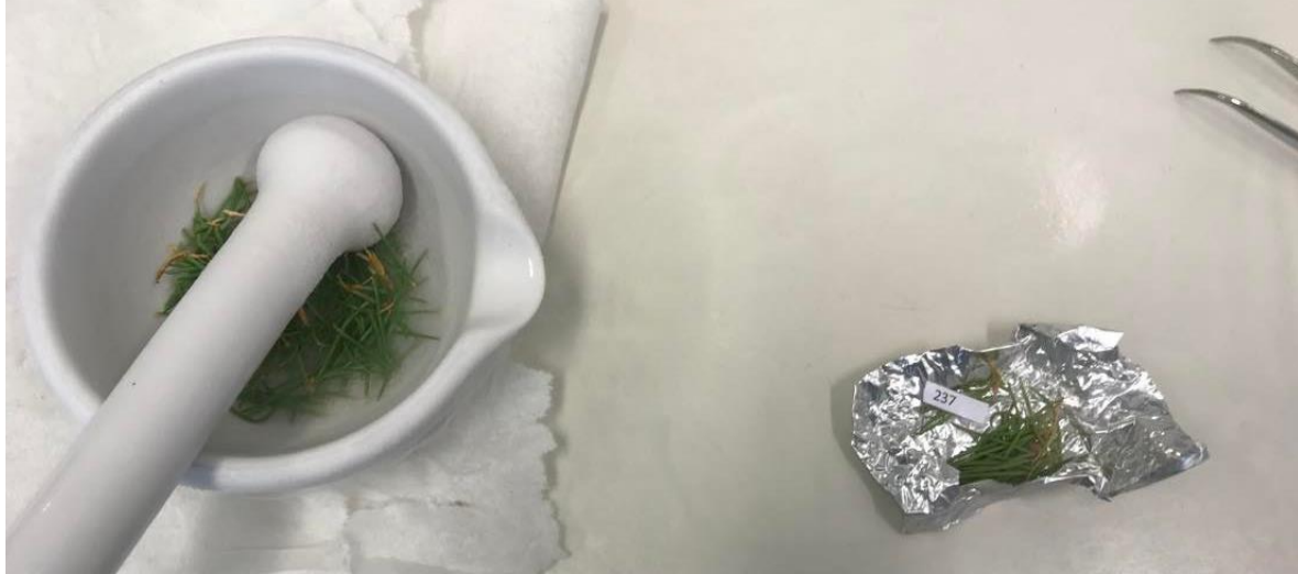
Fig 6: Pooled sample chilled with liquid nitrogen with mortar and a pestle before grinding.
