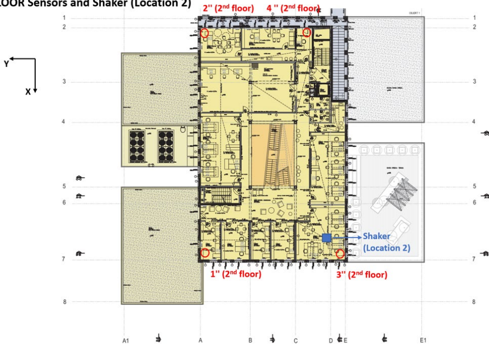
Figure 3-9: Location of 2 nd floor sensors and shaker.
