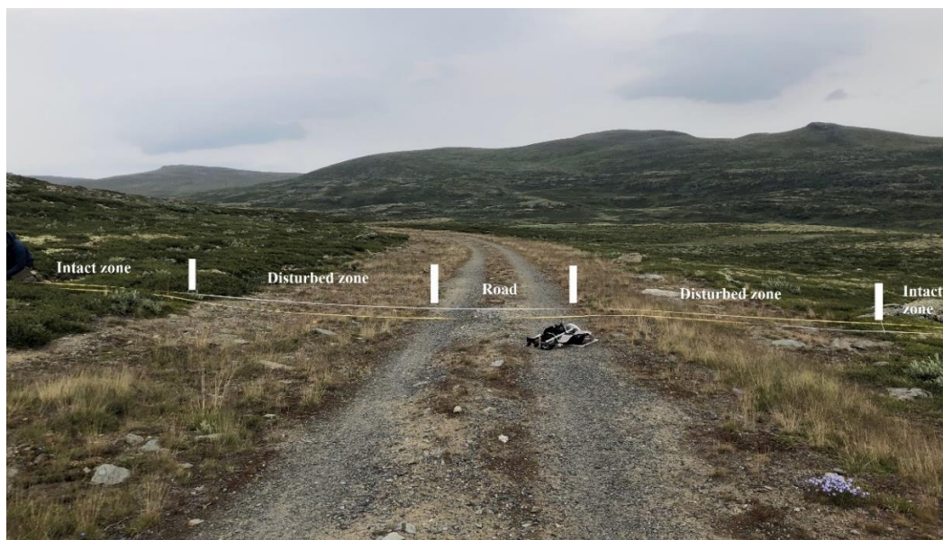
Figure 1: The transects are positioned across the road, and into vegetation (disturbed zone and intact zone, respectively) on both sides of the road.
