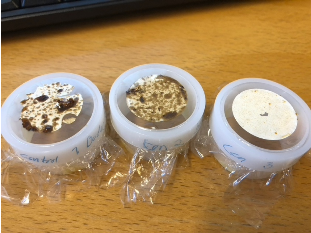
Figure 3.3: Examples of filters on \mu -XRF sample cups. The photo also illustrates the difference in digestion efficiency between samples. Photo: Ole-Johan Næss Holm
