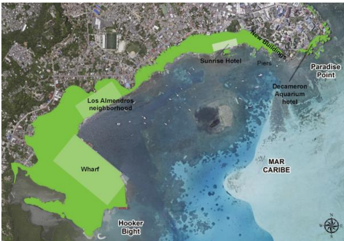
Figure 5: area reclaimed from the sea (green) in the service area of the Bay at North End. Adapted from Echeverry Hernández & Marriaga Rocha (2013).
