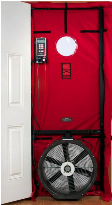
Figur 3.1 BlowerDoor system (The Energy Conservatory, u.å.-a)
