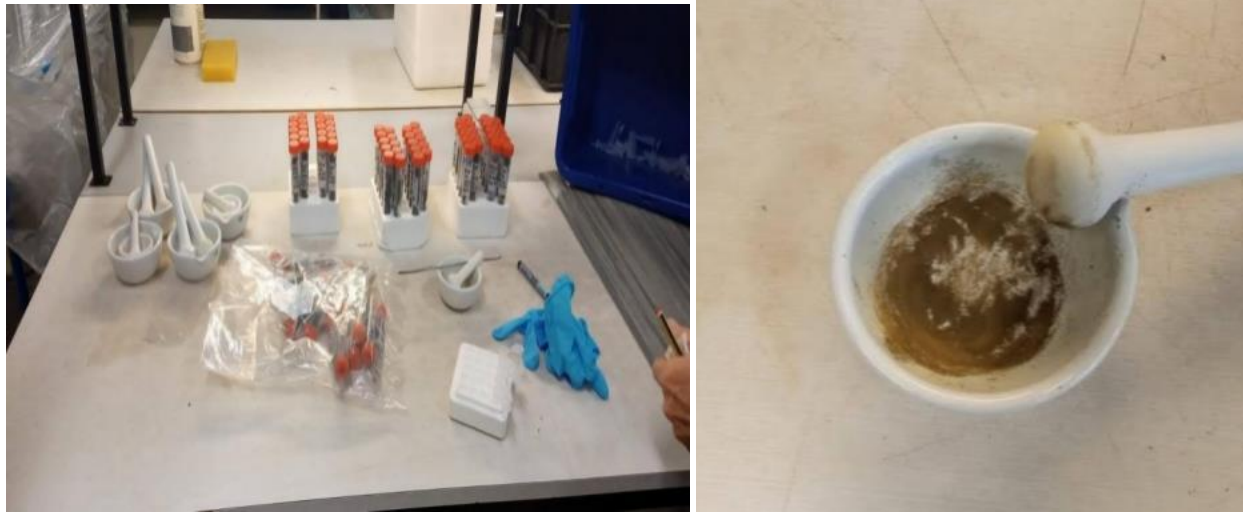
Figure 16: Showing pictures of mortars with pistils used in grinding the dried leaves and dried leaves in labelled 50ml tubes ready to be grinded for nutrient analysis (left), powdered sample after grinding (right). Photo: Gifty Kodua
