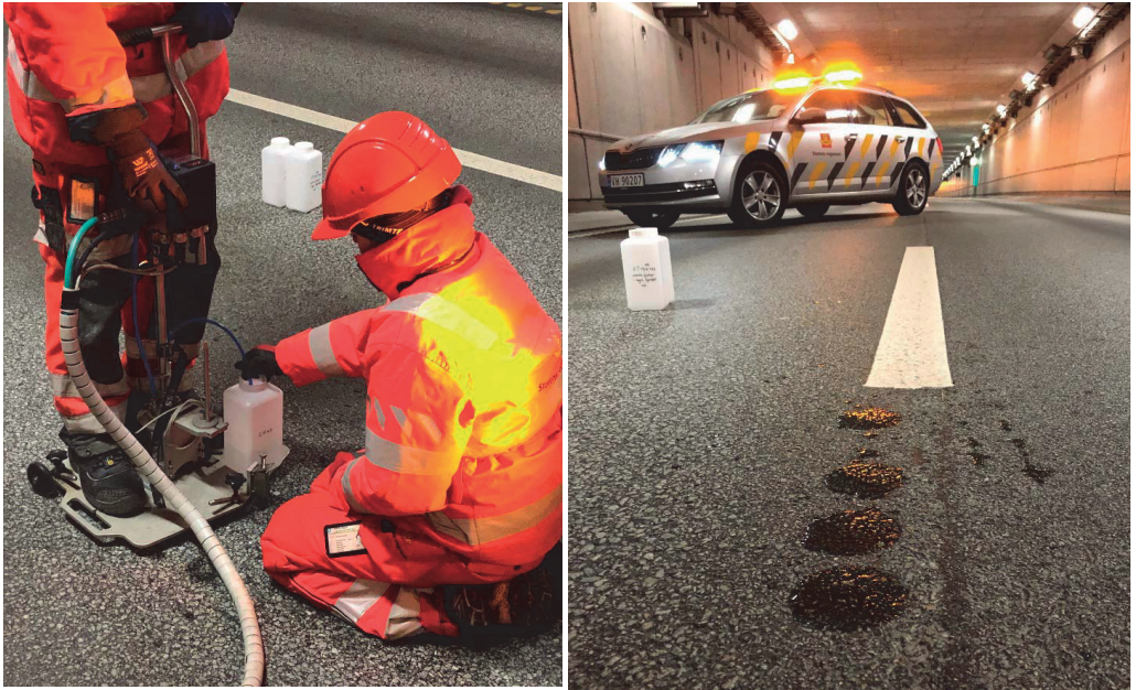
Figure 7. Sampling of tunnel road dust in the Smestad tunnel (Oslo, Norway) using the Wet Dust Sampler (left image: WDS; Lundberg et al. (2019)). Four consecutive areas were sampled for each location, leaving a wet stain on the road surface (right image). Sampling method is described in detail in Paper IV (Photos: E. Rødland)
