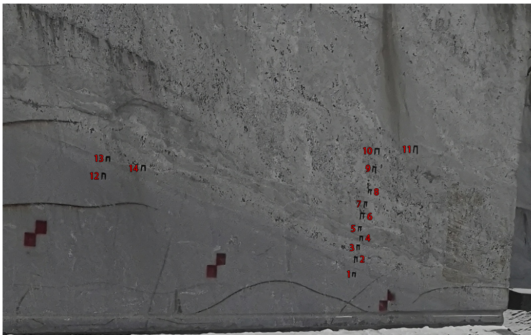
Figure 13: Labeling of the spots scanned with the XRF in the initial exploration of the quarry
