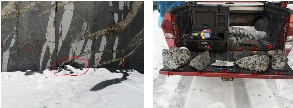
(a) The area from which the samples got collected (b) The samples collected from the wall
