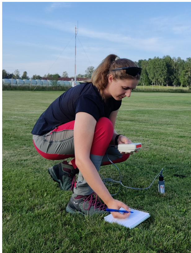
(b) Noting down readings from the HH2 meter when taking measurements with the ThetaProbe. Photo: Private.
