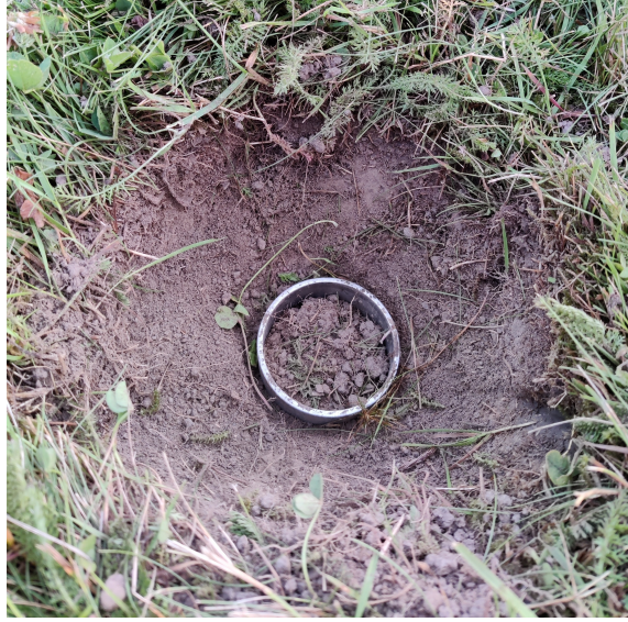
Figure 10: A 100 cm 3 cylinder used in the field for gathering soil samples for the volumetric method.
