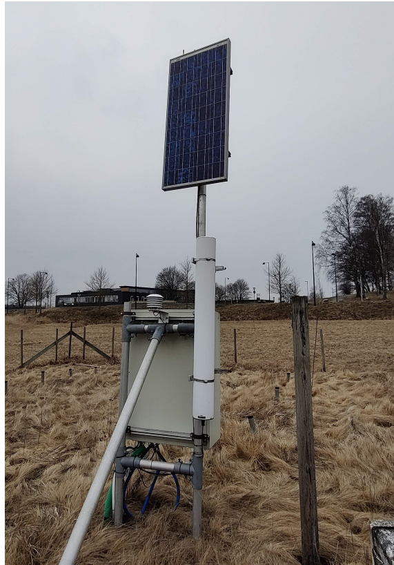
Figure 14: The CRS-2000/B sensor (COSMOS) installed in Kjerringjordet. Photo: Ida Lunde Naalsund.
