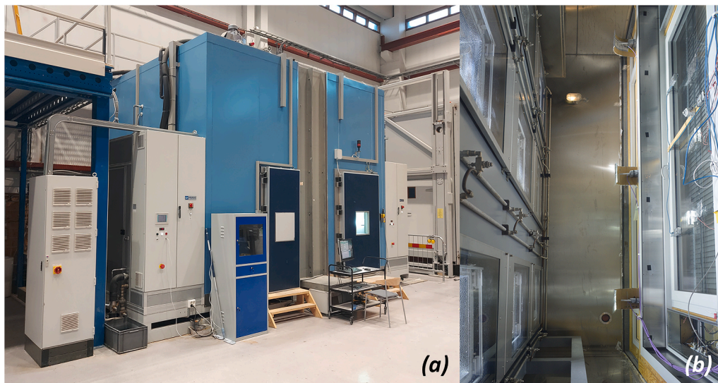
Fig. 4. The climate simulator facility (a); the DSF test sample placed in the climate simulator (b) - view from the outdoor chamber with the solar simulator's lamp array on the left-hand side of the picture and the DSF mock-up on the right-hand side of the picture.
