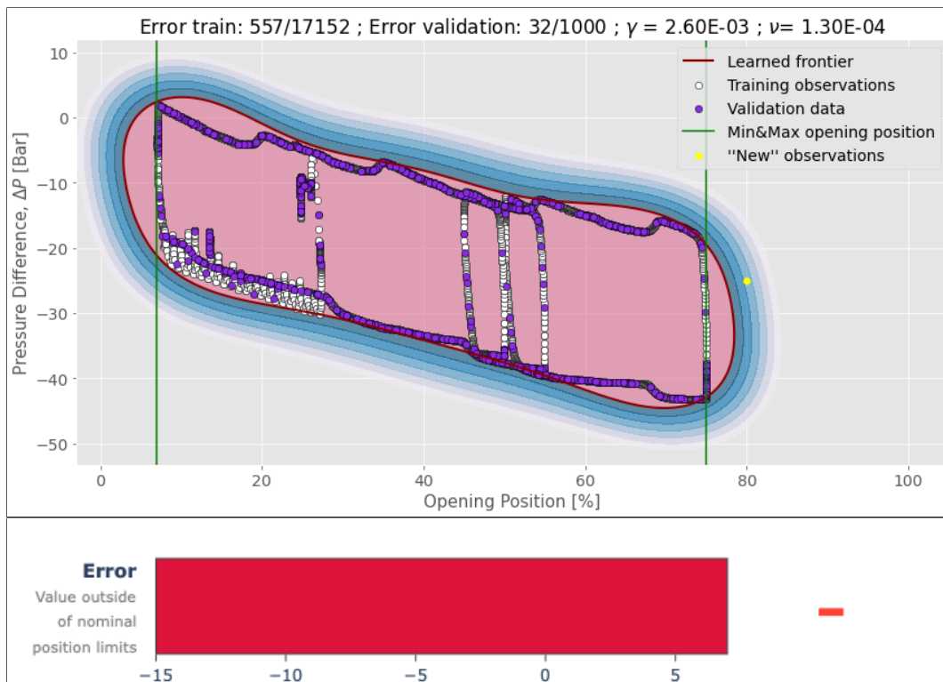
FIGURE 5.21: One Class SVM classification for pressure difference with KPI visualised as a bullet chart, when new value is out of nominal position boundary.
