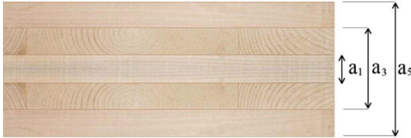
Figure 3.19: Thickness definition by Follesa et al. (2013).
