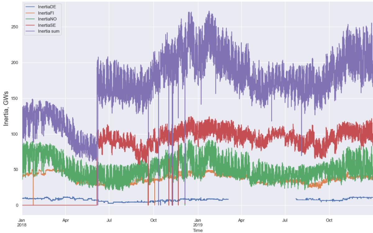
Figure 3.1: Inertia as stored by Innsikt. The figure displays the kinetic energy in GWs for Denmark (blue), Finland (yellow), Norway (green) and Sweden (red). The purple curve is the aggregated total.
