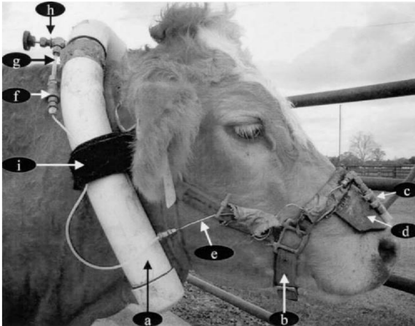
Figure 2.3 Methane collection equipment as worn by a grazing cow: (a) collection canister; (b) halter; (c) filter inlet connected to capillary tubing; (d) leather muzzle protector; (e) stainless steel capillary tubing attached to halter; (f) quick-connect coupling of tubing to canister; (g) Teflon tubing between shut-off valve and quick-connect to capillary tubing; (h) shut-off valve on canister; (i) Velcro strip to anchor canister to halter (DeRamus et al., 2003).
