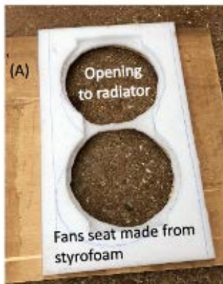
(A) Fans seat made from styrofoam to concentrate air flow through opening to Radiator. (B) Fans installed on styrofoam seat and surface board.
