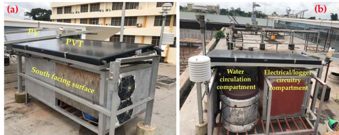
Figure 2. Photovoltaic-thermal (PVT) showing: (a) south facing surface and cooling fans for radiator (left); (b) north facing face with water circulation compartment and electrical/logging circuitry compartment (right).
