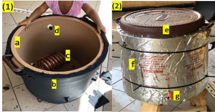
Figure 3.5: Some details of thermal storage vessel showing: (a) the thermos vessel, (b) armaflex insulation, (c) heat exchanger, (d) spout for transducer insertion, (e) non modified lid, (f) thermal resistant foil cover and (g) manual valve
