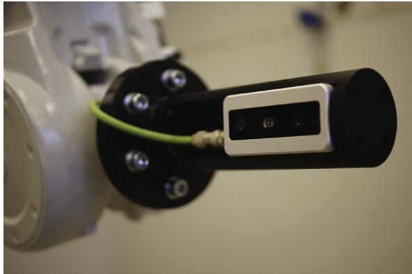
Fig. 8. Camera attachment to the robotic arm.
